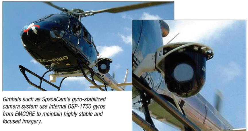
Gimbals such as SpaceCam's gyro-stabilized camera system use internal DSP-1750 gyros from EMCORE to maintain highly stable and focused imagery.
